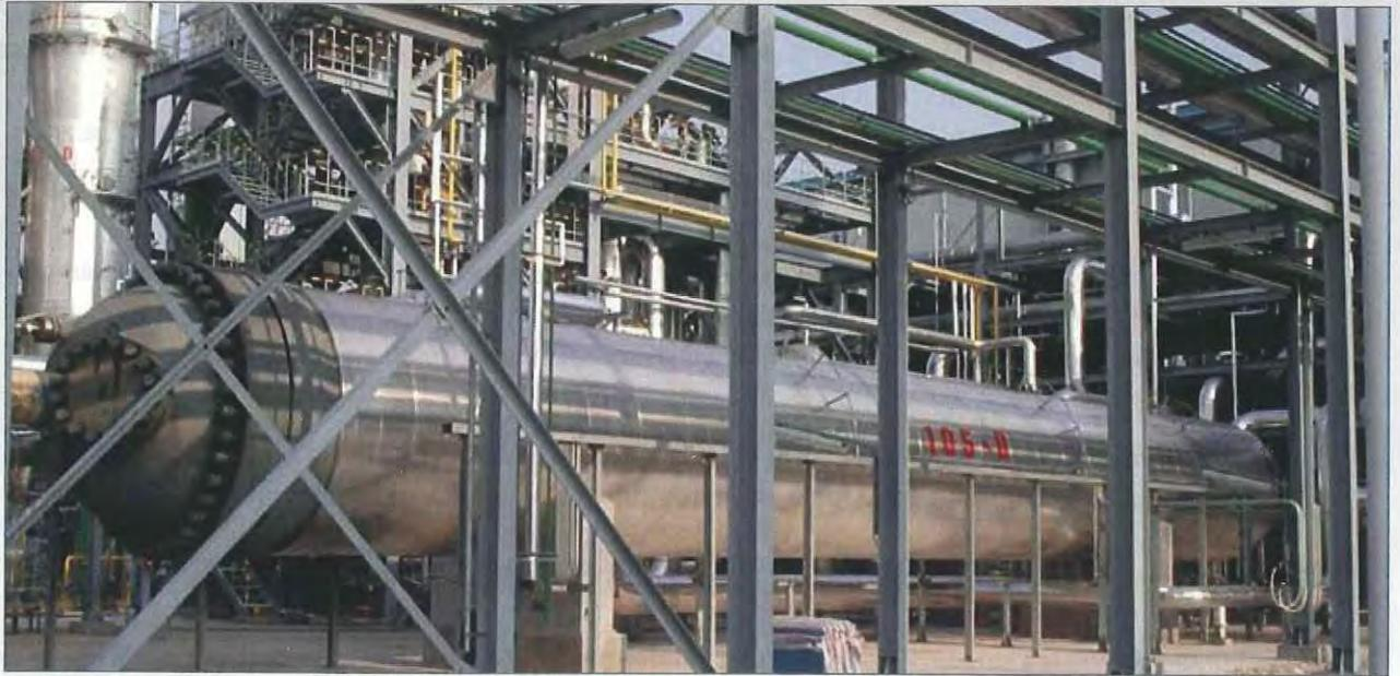
For conventional magnetite synthesis loops, KBR offers its horizontal ammonia synthesis converter. Inter-stage coolers between the catalyst beds provide for maximum conversion and heat recovery.
