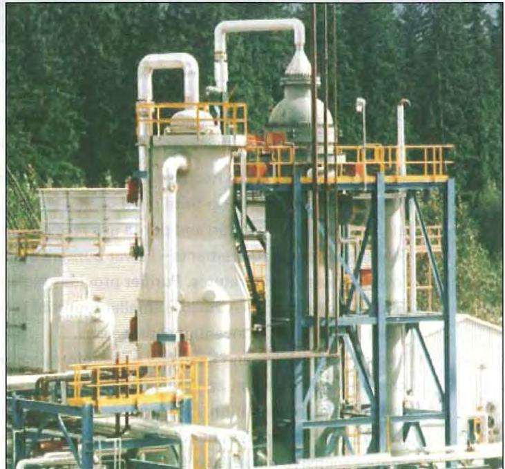
KRES Autothermal Reformer (left) and KRES Exchanger (right) as installed at an ammonia plant in British Columbia, Canada
