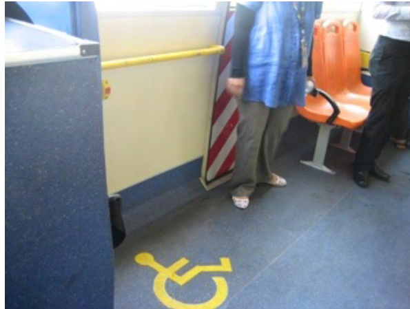
Photo 2-5-12 space for wheelchair users on the ultra low-floor bus
