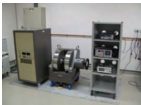
Photo 1 Standard magnetic field generation system (Tamakawa Works Co. Ltd.)
