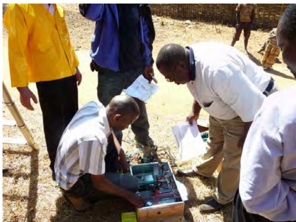
Photo 1 Preparation of equipment to measure actual load of the TC.
