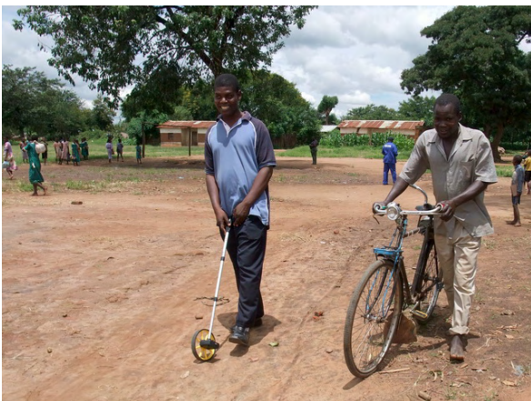
Photo 5 B/D using wheel measure (conventional method)
