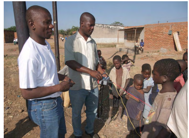
Photo 4 Measurement of earth resistance by DOE
