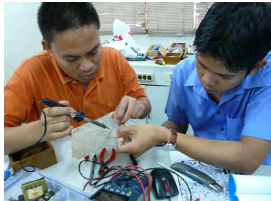
Fabrication of ELC Plate
