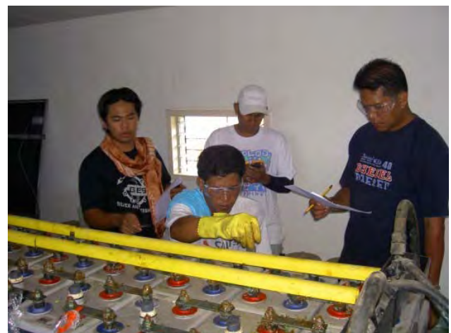
Measurement of specific gravity of battery
