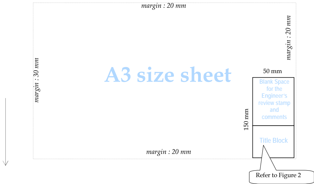
Format of the Contractor's Drawings
