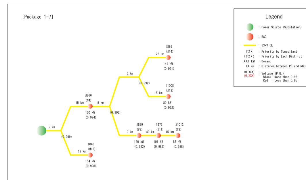
DL System at Kasempa SS Feeder 1 (Package 1-7)
