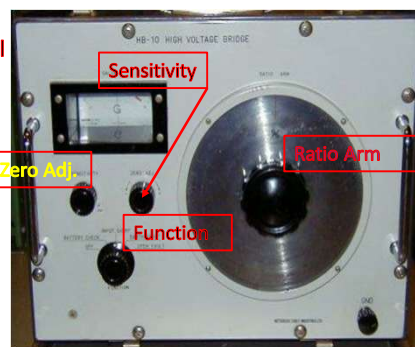
Bridge circuit (analog type)
