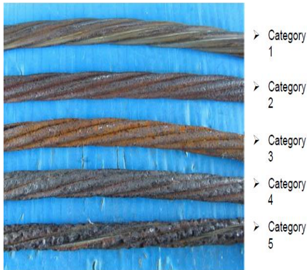
Figure 10 Steel conductor condition/corrosion categories
