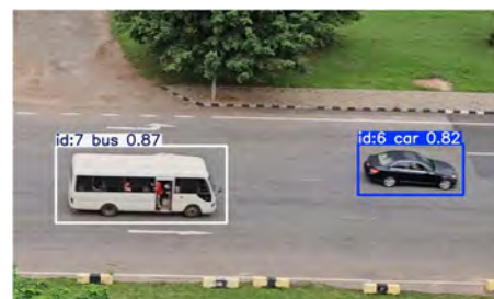
Figure 6.2.2 AI Traffic Count Survey Test Results
