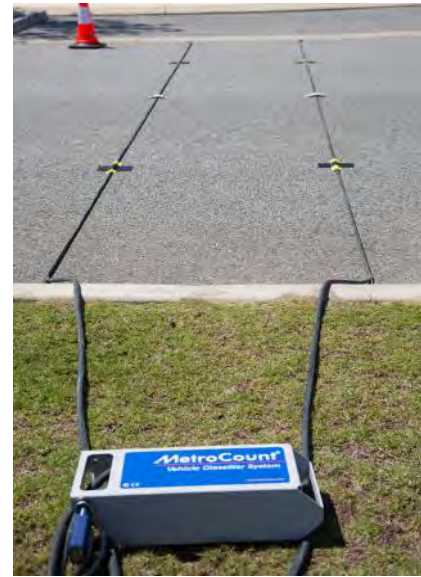
Figure 6.2.1 Vehicle Detection Sensors Installed on the Road (Metrocount)
