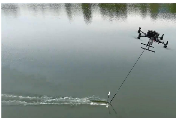
Photo 2.2.6 Work at Site with Single Beam Sonar
