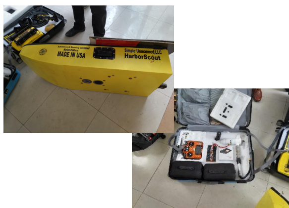
Photo 2.2.4 Radio Control Boat for Surveying the Riverbed
