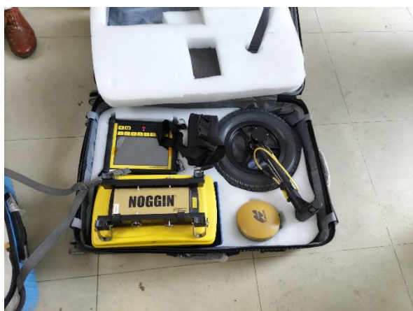
Photo 2.2.1 Portable Ground Penetrating Radar
