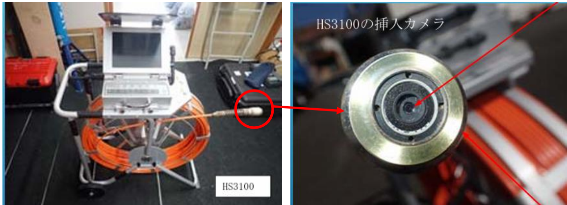
Figure 7 CCD camera for borehole monitoring
