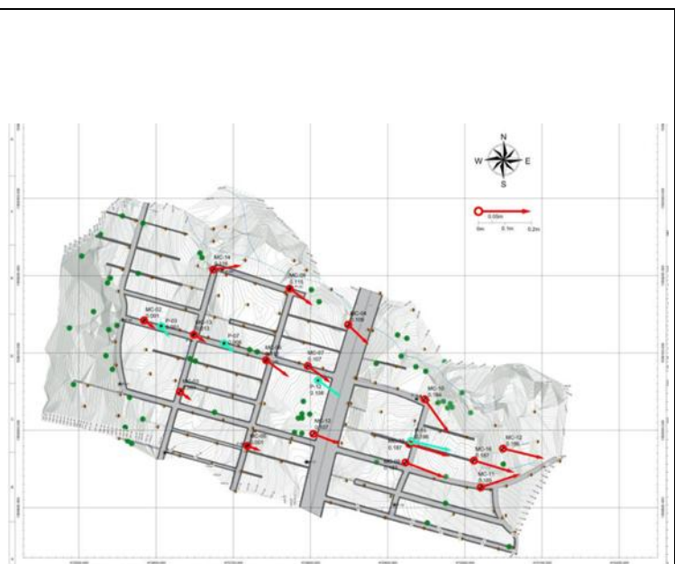
Figure 1.9 Illustration of Observation Points Monitoring Results (Movement Vectors) on Jose Angel Ulloa 2)
