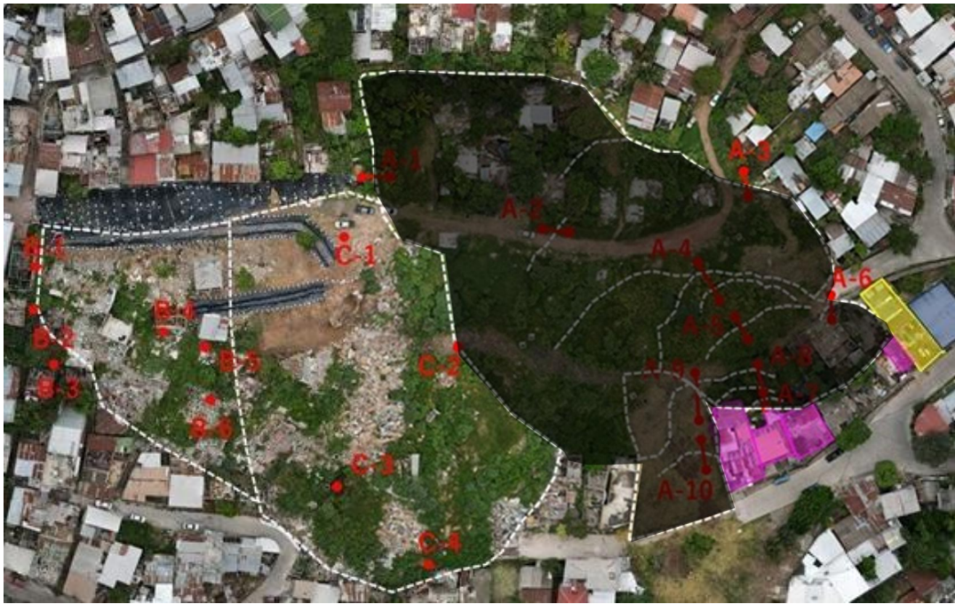
Figure 2-2 Monitoring point of surface measurement in La Guillen
