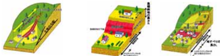
Debris flow Slope failure/ Rock fall Landslide
