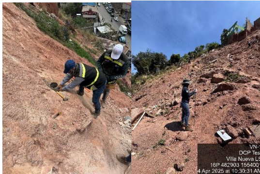
Figure 33 Sampling of undisturbed sample. And Simplified Dynamic Cone Penetration Tests
