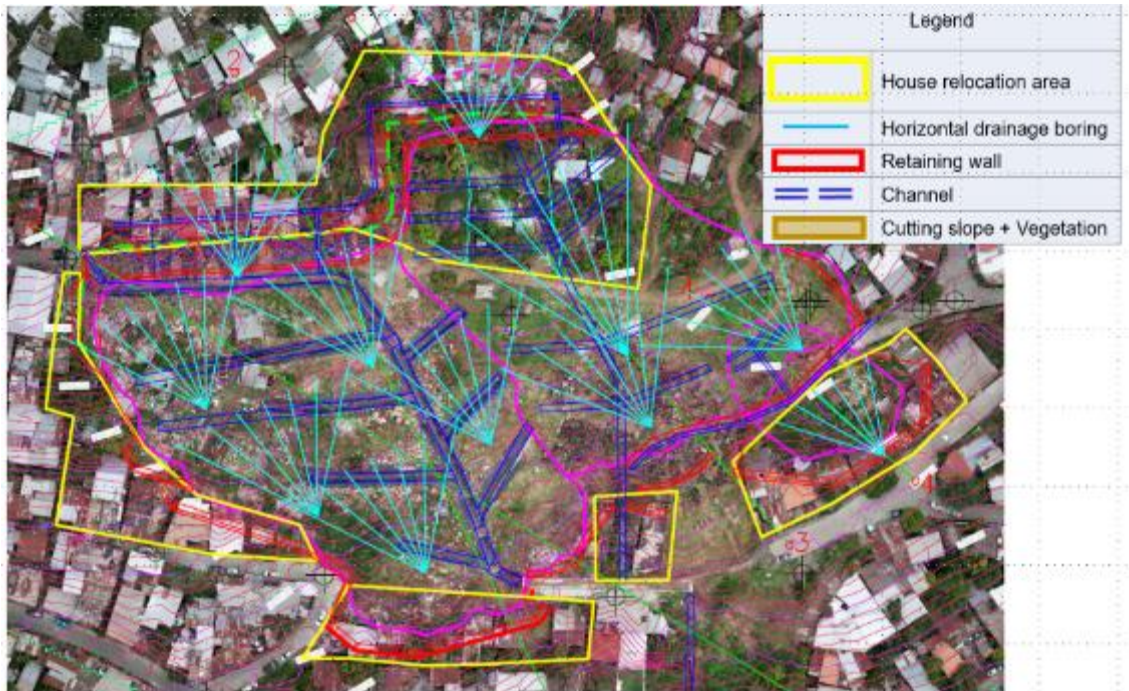
Figure 79 Plan view of the countermeasure work (preliminary design) and the range of required houses relocation of residences
