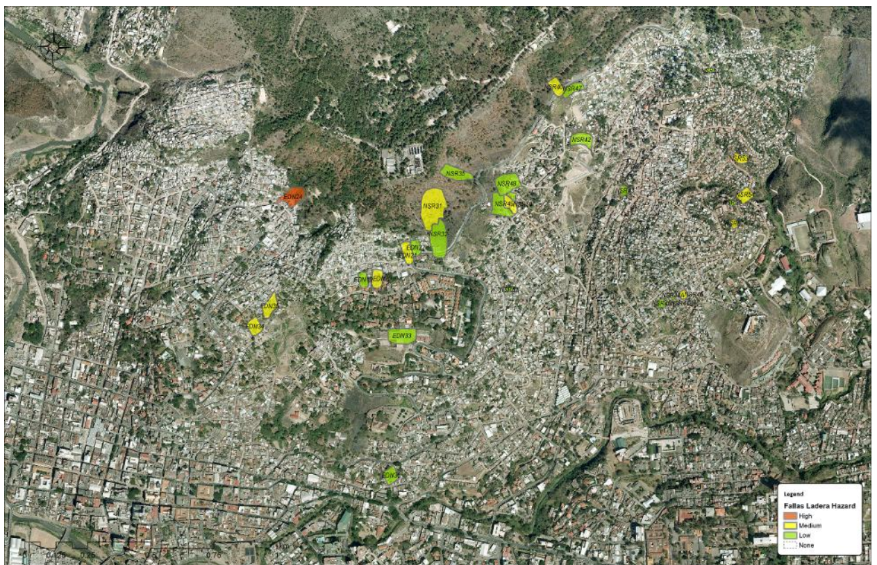
Figure 190 Slope failure/rockfall hazard map
