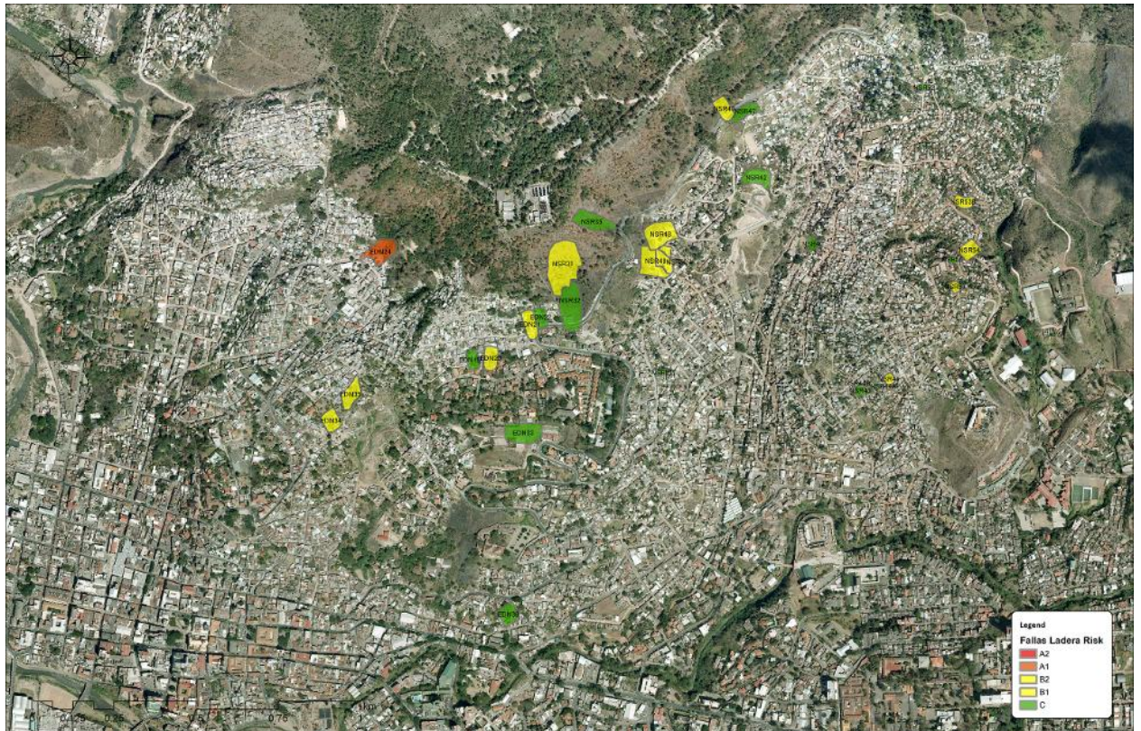
Figure 191 Slope failure/rockfall risk map
