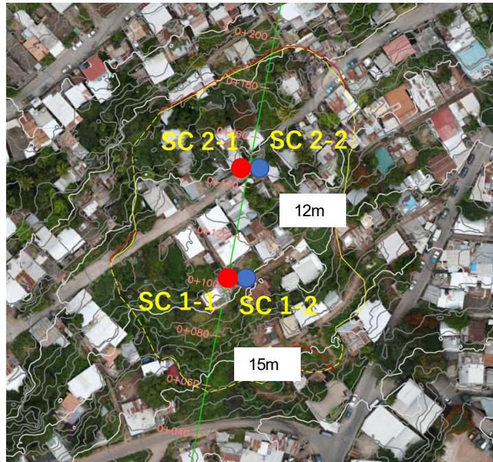
Figure 202 Monitoring plan in the Suazo Cordova landslide site
