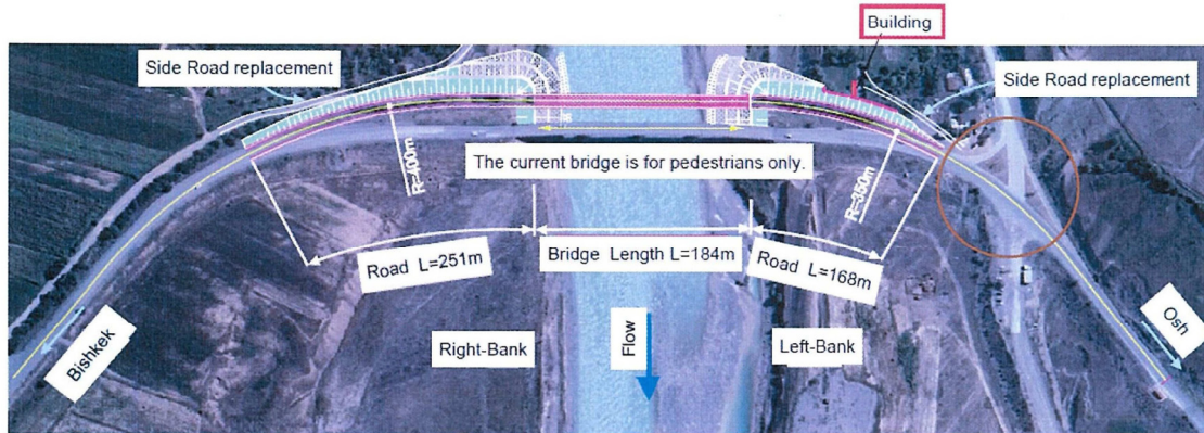
Figure-1: Scope of project
