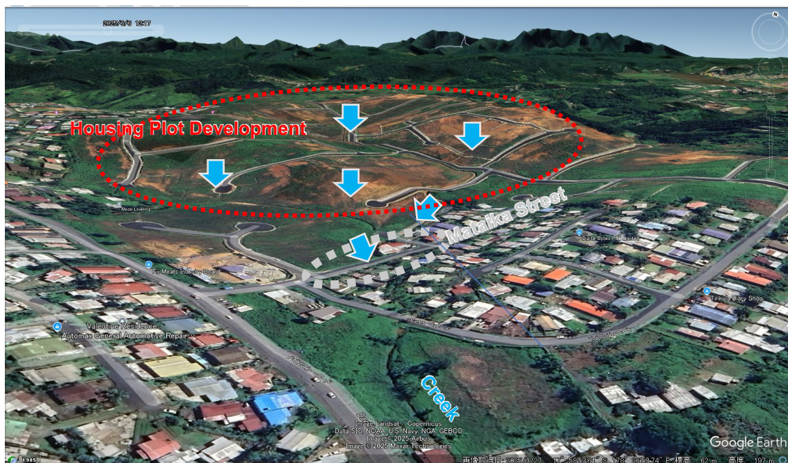
Figure 3-16 Example of Impact of Development on the Downstream Flooding
