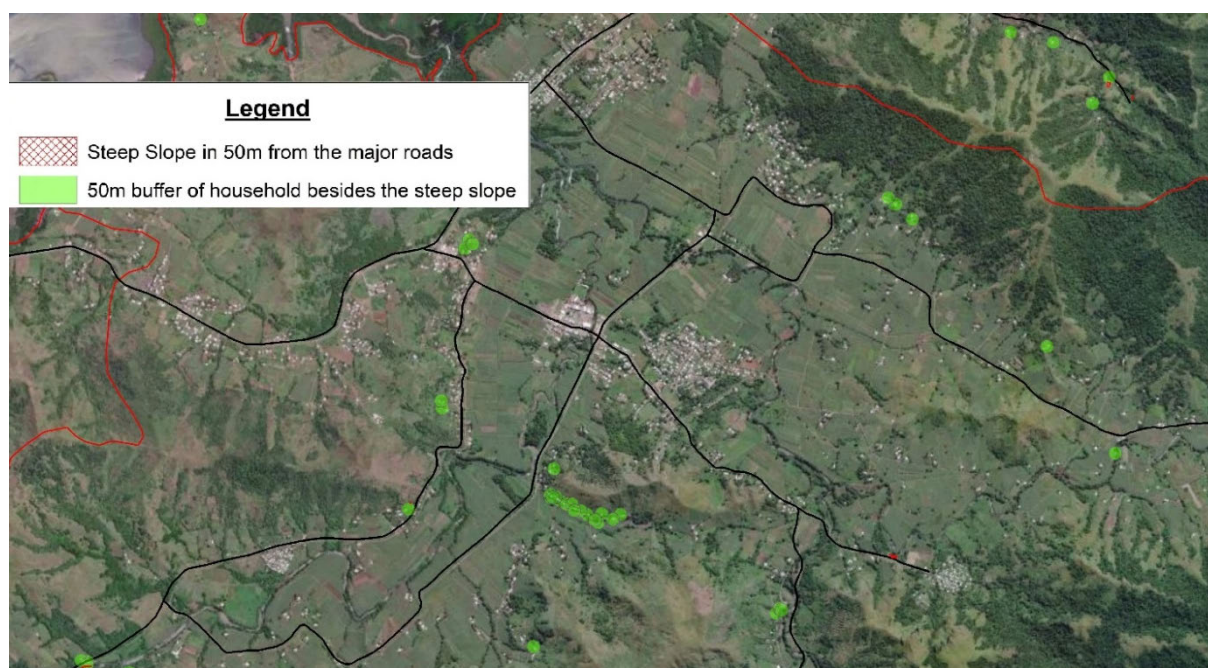
Figure II-6 Hazard Assessment of Steep Slope Collapse in the Rakiraki River Basin
