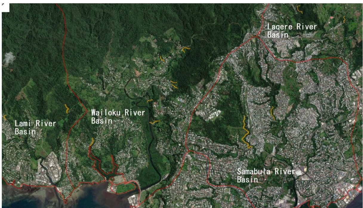
Figure II-5 Hazard Assessment of Debris Flow in Suva area (risk areas are orange-colored areas on the map)
