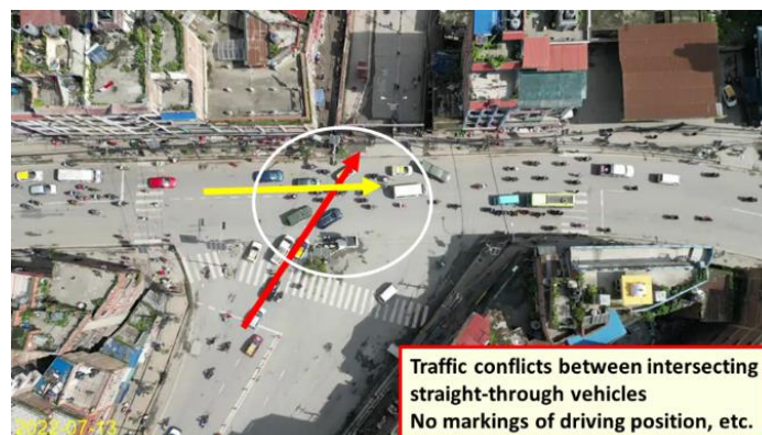
Figure 5-2 : Example of Video Analysis from Drone Photography (Traffic Conflicts Between Intersecting Straight-Through Vehicles)
