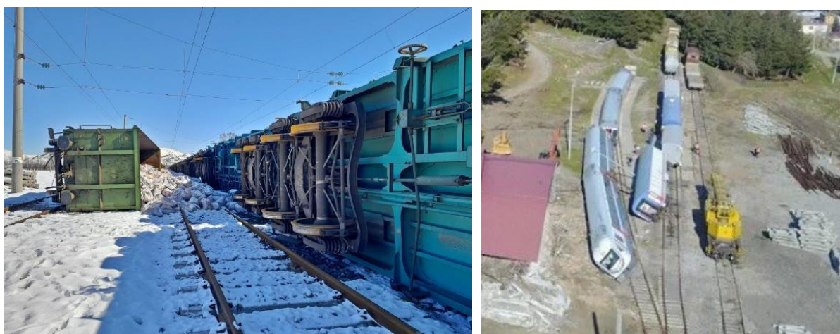
Figure 6-2 Derailment Due to the Earthquake (Left: Gölbaşı Station, Right: Fevzipasa Station)
