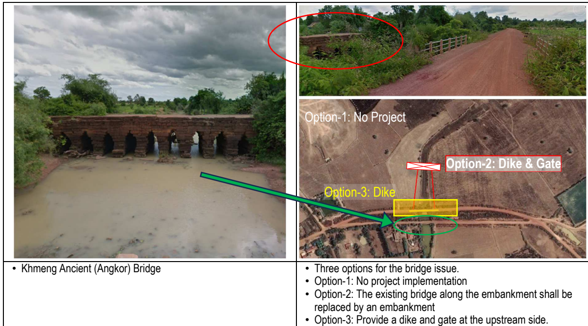
Figure 6.3.8 Rehabilitation Plan of Khmeng Ancient Bridge
