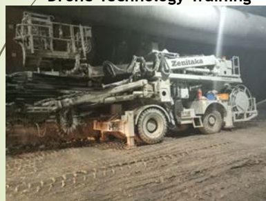
Drill Jumbo (Boring and Rock Bolting)
