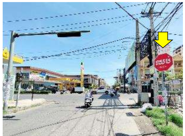
Figure 7.22 Examples of Inappropriate Traffic Signs (Stop Signs at Signalized Intersections)
