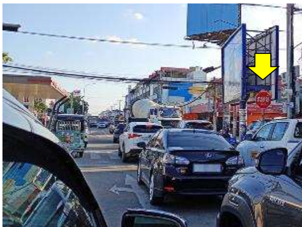
Figure 7.22 Examples of Inappropriate Traffic Signs (Stop Signs at Signalized Intersections)
