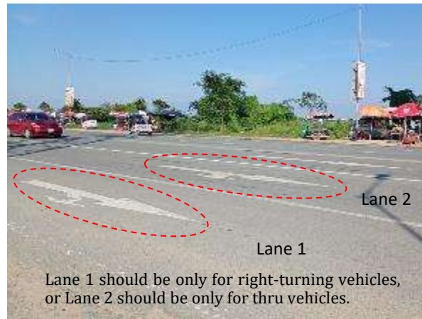
Figure 7.23 Example of Inappropriate Road Marking near AEON III
