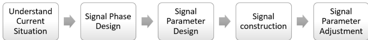
Figure 4.1 Flowchart of Signal Improvement Work
