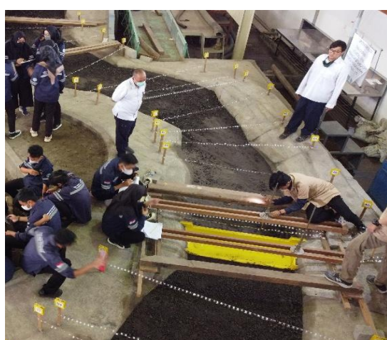
(Verification of sediment deposition process in a meandering section of a Sabo dam, 2021)
