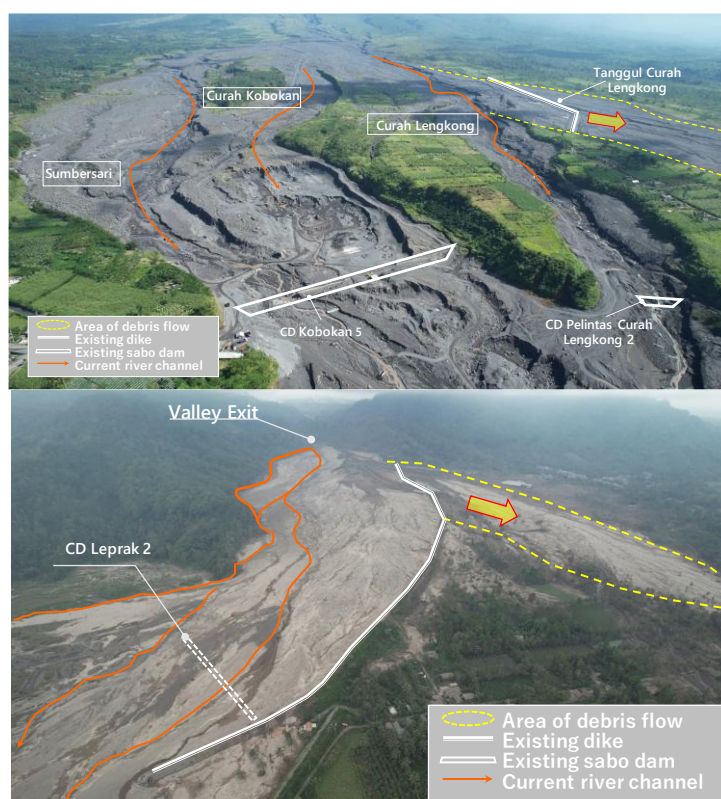
Figure 3-18 Sediment disaster status in S2 and S4 (above: S2 area, bottom: S4 area)
