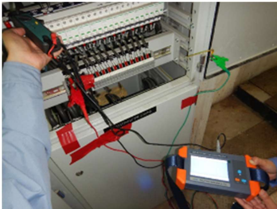
Figure3: DC circuit ground fault detection
