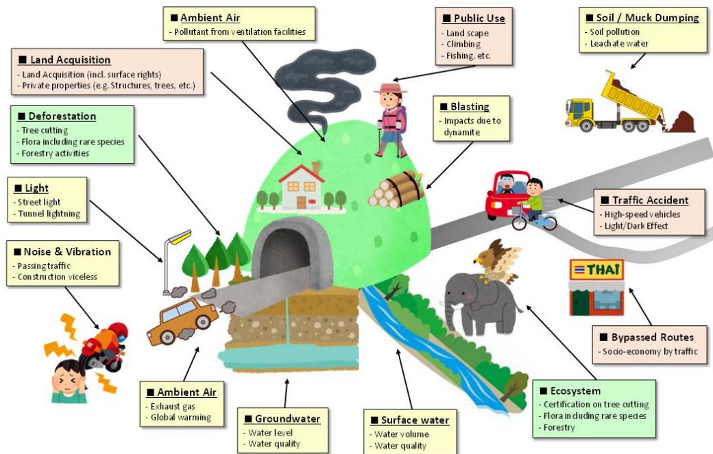
Major Possible Impacts on Environmental and Social Considerations Caused by a Tunnel Project in Mountainous Regions
