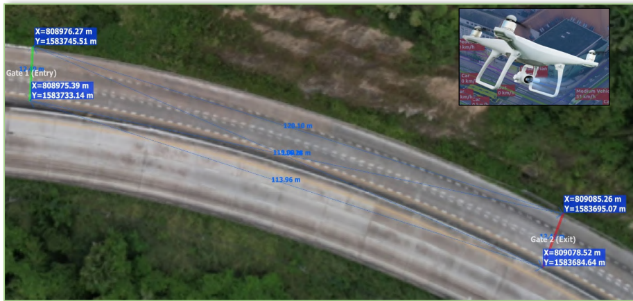
Figure 5.3.79 Vehicle Trajectories Analyzed by AI Image Processing
