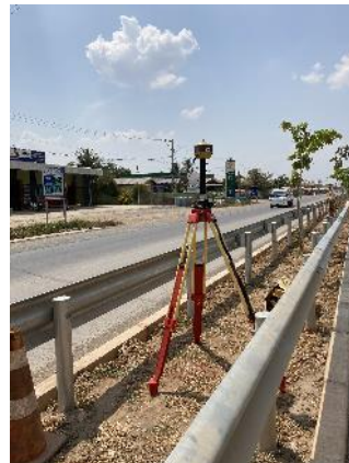
Figure 2-7 Static Survey (Left: Survey for RTK base station / Right: Survey for set up mmGPS equipment)
