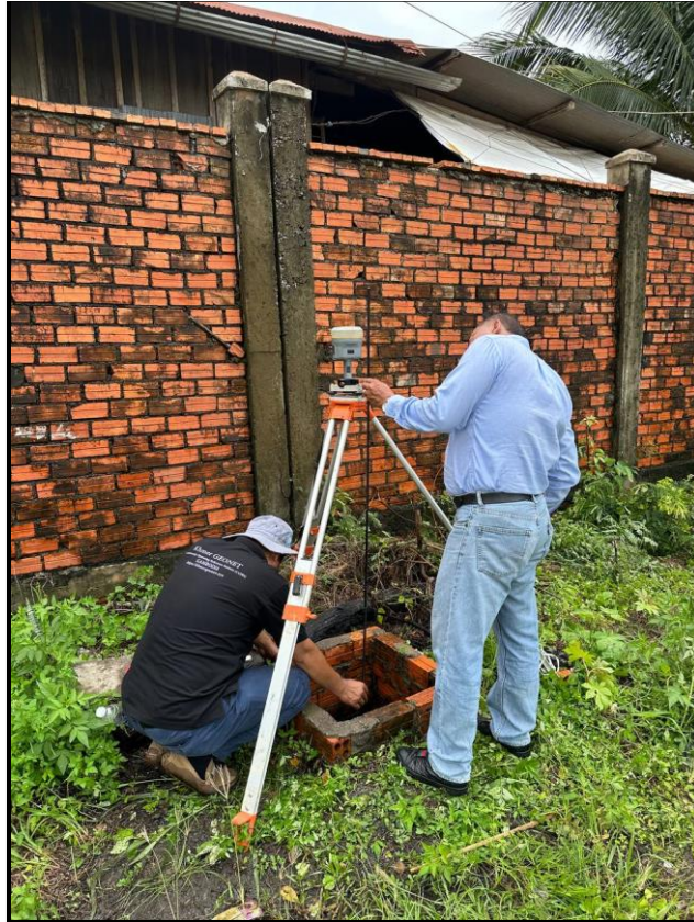
Figure 2-1: Trimble R10 receiver setup on national control point "5"
