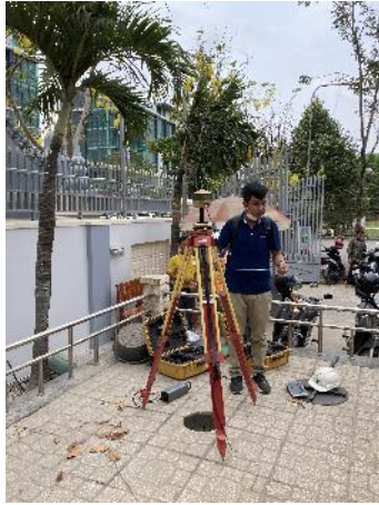
Figure 2-9 Comparison of N-RTK vs RTK survey (Pictures are setting for RTK)
