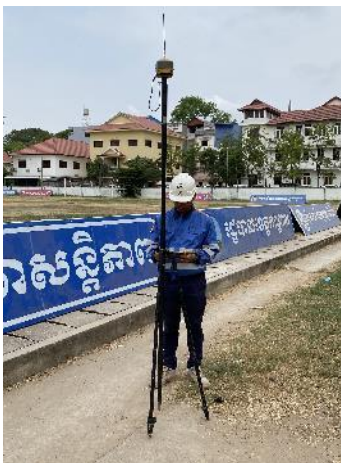
Figure 2-10 Comparison of N-RTK survey vs RTK survey (Pictures are collecting data on survey points)
