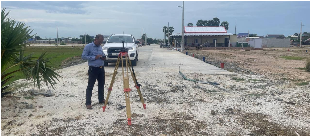
Figure 2-17: Tripod Setup for boundary survey
