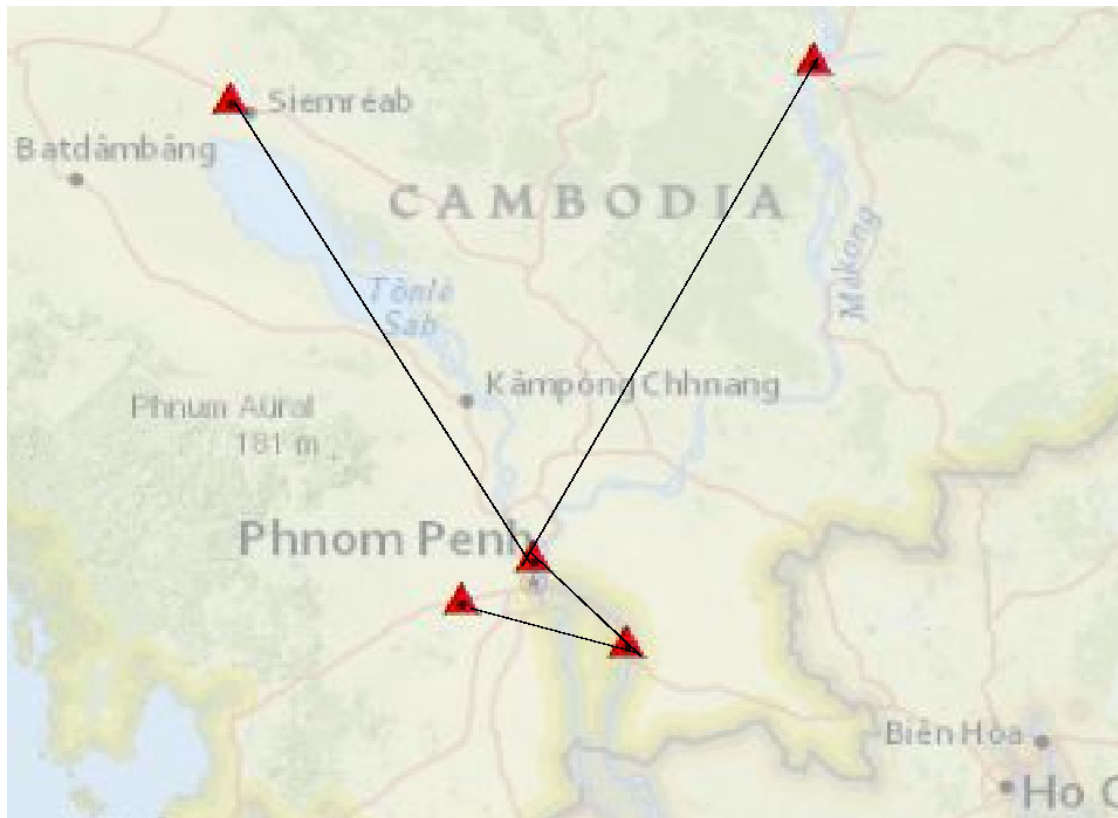
Figure 4 Applicable area and CORS distribution of Khmer GEONET
