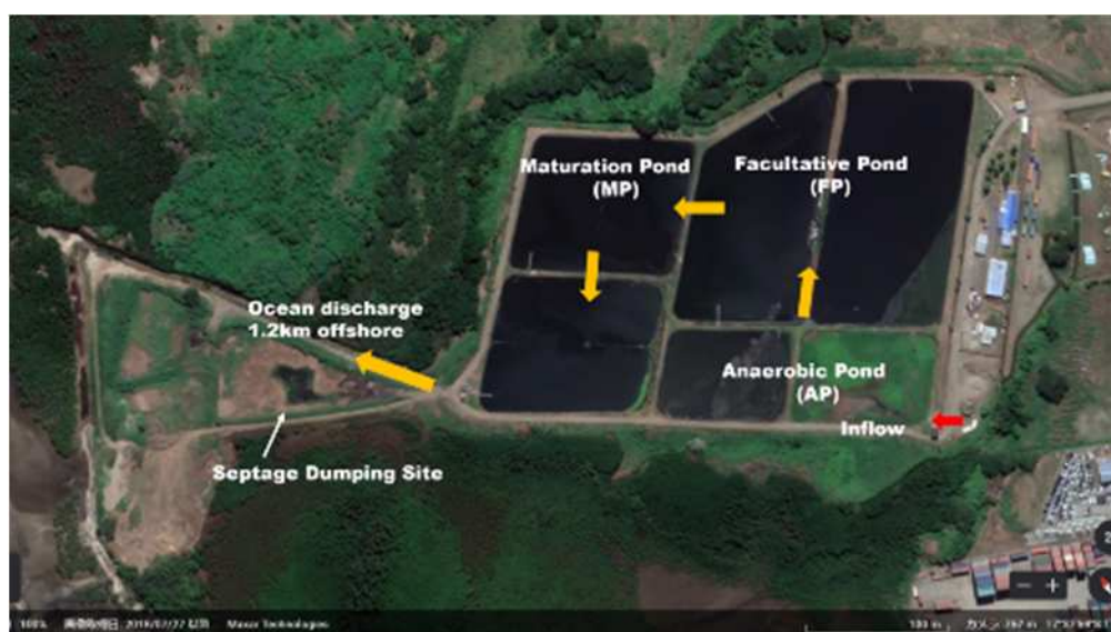
Figure 2-1.2 Layout of Facilities in Natabua WWTP
