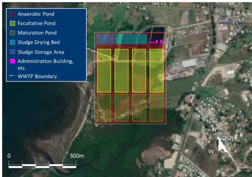
Figure A4-4.1 Stabilization Pond: 10,000 m 3 /day Model Footprint
