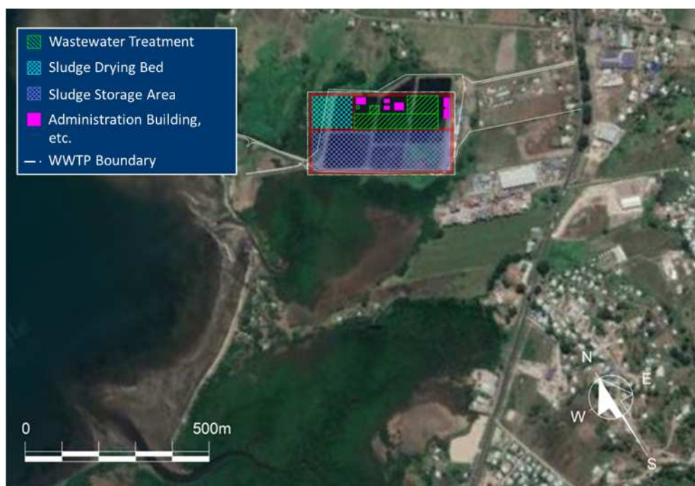
Figure A4-4.5 Oxidation Ditch: 10,000 m 3 /day Model Footprint
