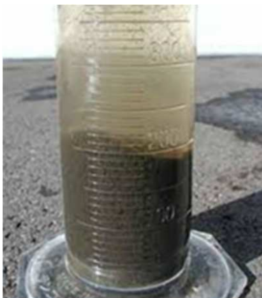
Figure S4. 3-2 SV Measurement at Navakai WWTP
