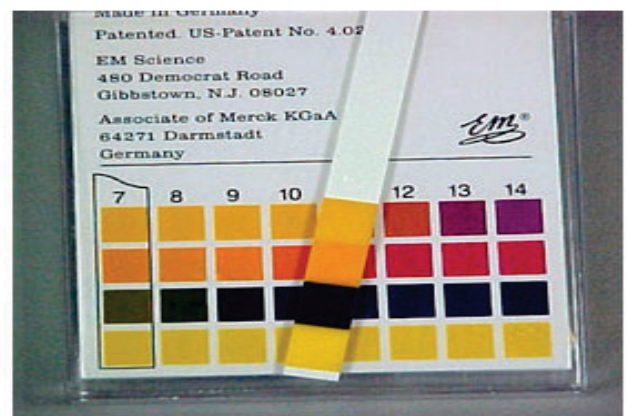
Figure 16: Reading pH value after adjustment (9 pH) (Step 4)
