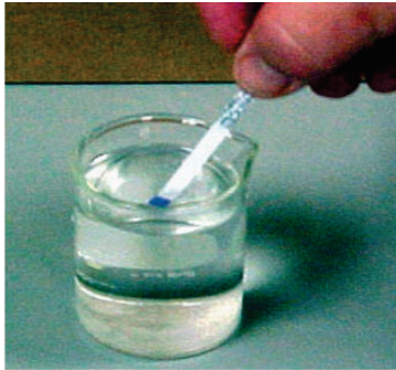
Figure 13: Dipping indicator strip into make-up water (Step 2)
