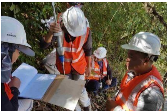
Conduct of Handy Dynamic Cone Penetration Test by C/P Trongsa regional office jurisdiction (November 6, 2019) (Source: JET)
