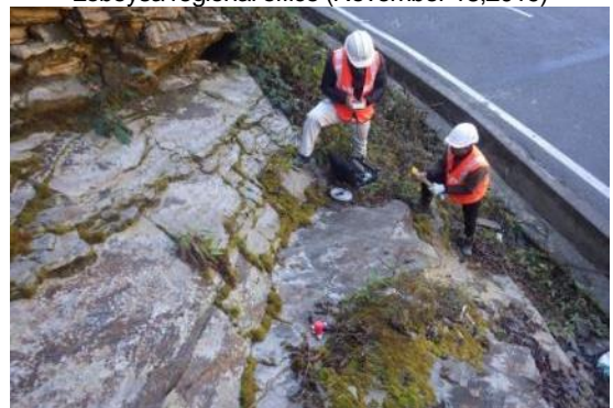
Measuring a Vp velocity using simplified method by C/P Lobeysa regional office jurisdiction (November 28, 2019)
