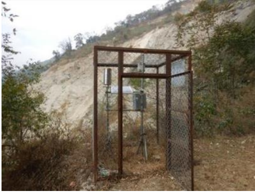
Output 1: Rain gauge and local communication base station (Apr 26, 2019)
