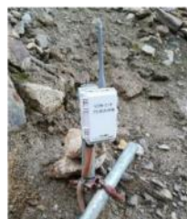
Figure 3.2-15 Deployment of base stations and ground surface tilt sensors (Razhau)
