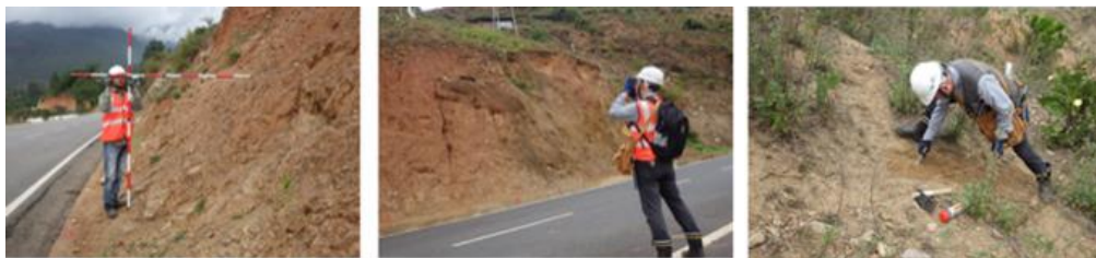
Photo 3.3-25 Simplified surveying (left: pole surveying, middle: surveying with distance meter, right: soil hardness measurement)
