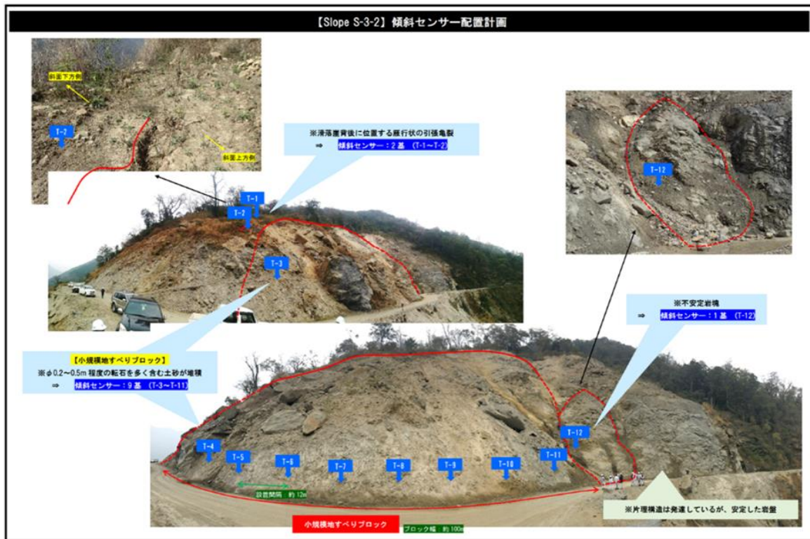
Figure 3.2-14 Deployment plan of base stations and ground surface tilt sensors (Reotala, Tonsa office)
