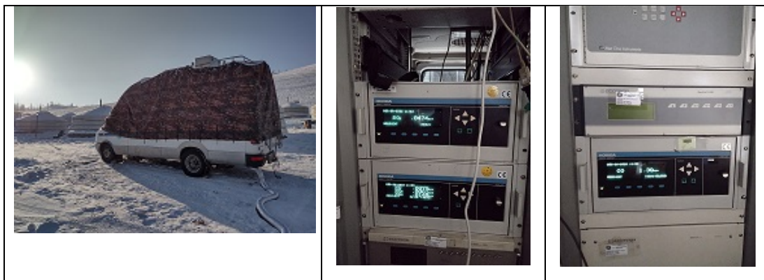
Photo 3-2-3 Air Quality Monitoring at Ger Campsite by Mobile AQMS
