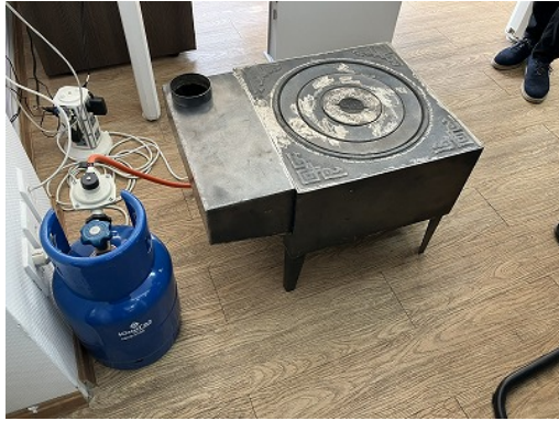
LP gas Ger stove Improved traditional coal Ger stove. Currently, gas consumption is high, and fuel efficiency needs to be improved.
