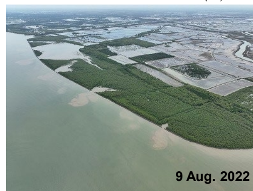
Protection Measure (Mangrove Plantation) at Fishpond (P4)
