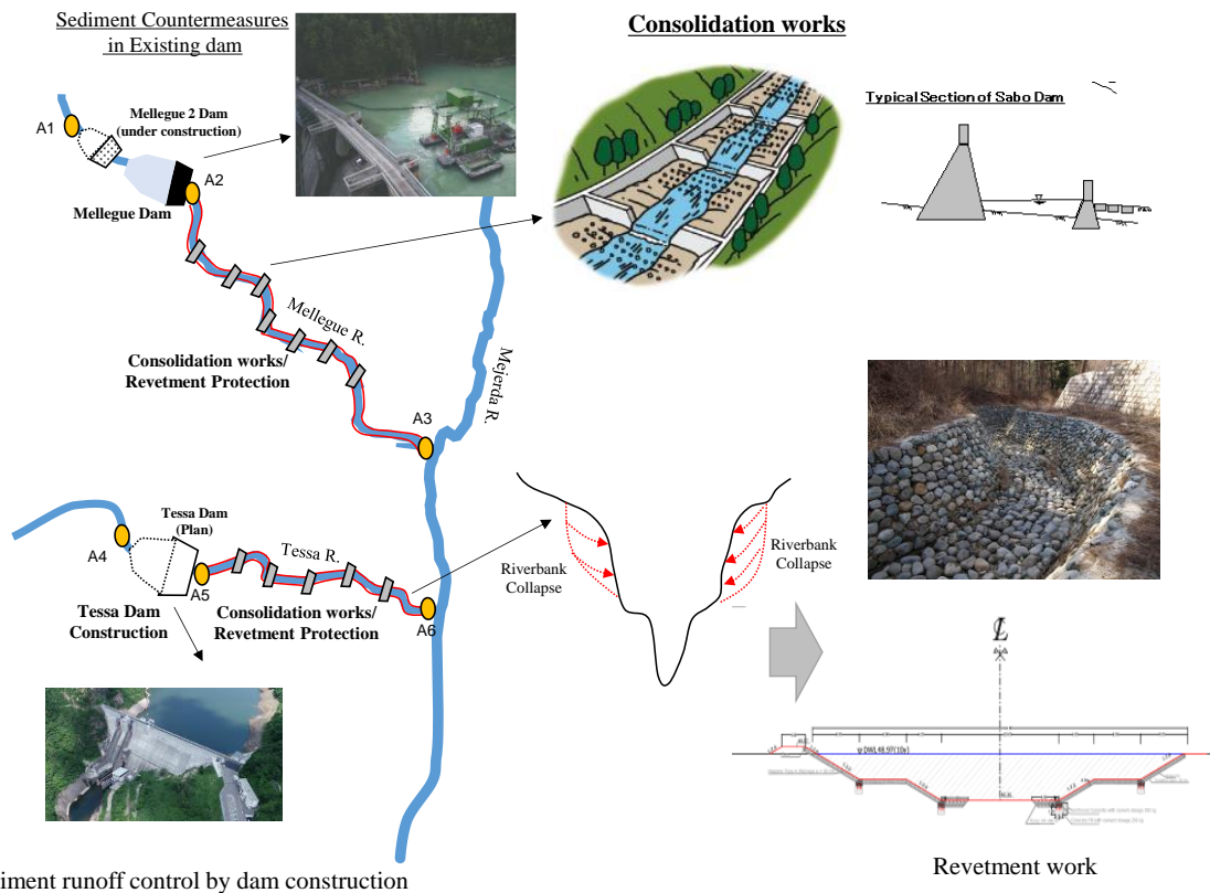
Figure 18-29 Countermeasures for Riverbank Erosion and Sediment Production inside Rivers
