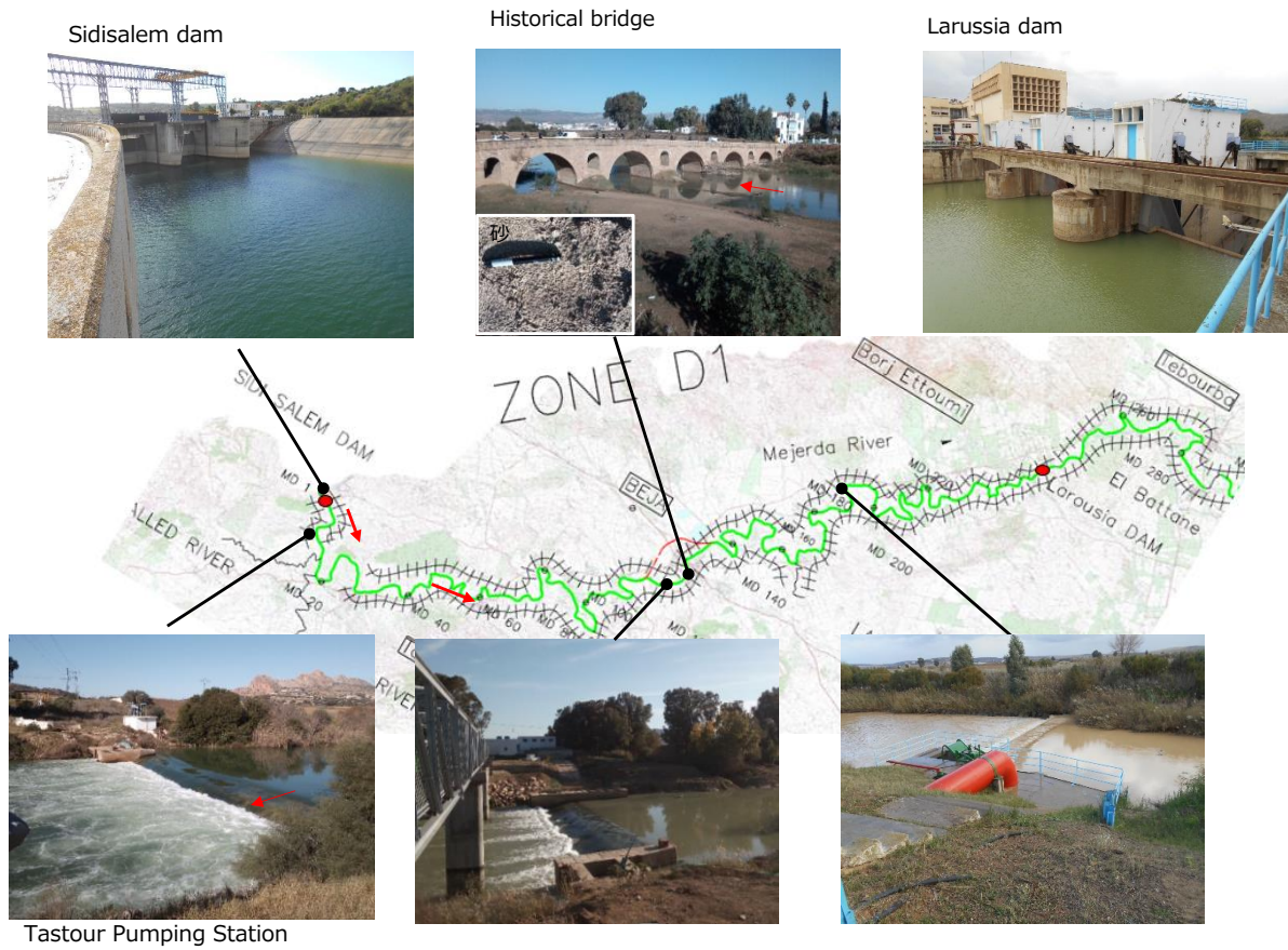
Figure 11-11 River Crossing Structures in D1 Zone
