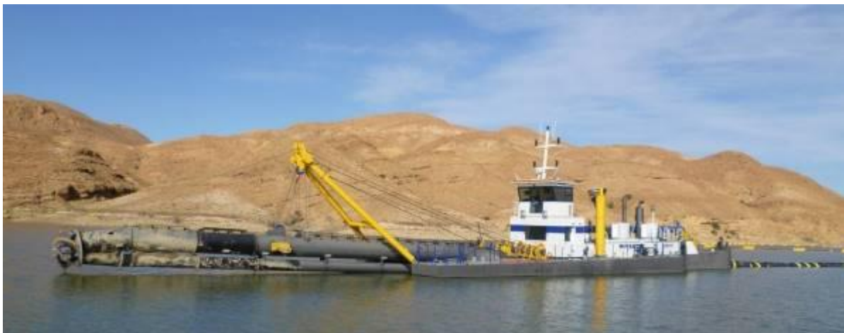
Figure 8-1 CSD500 with X-mas Tree Commissioned and at Work
