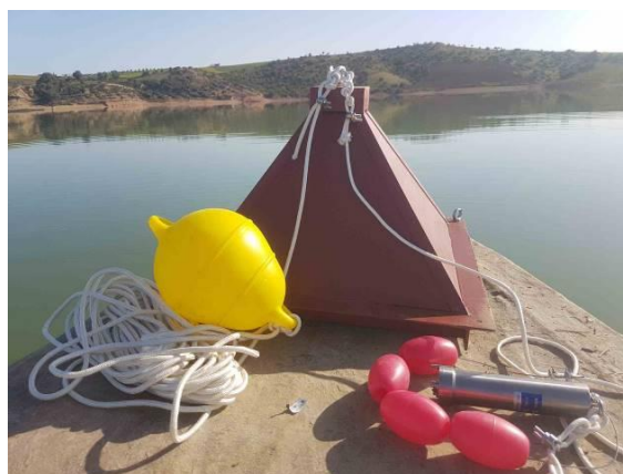
Figure 5-35 Equipment for Turbidity Survey Installed in the Dam Reservoir
