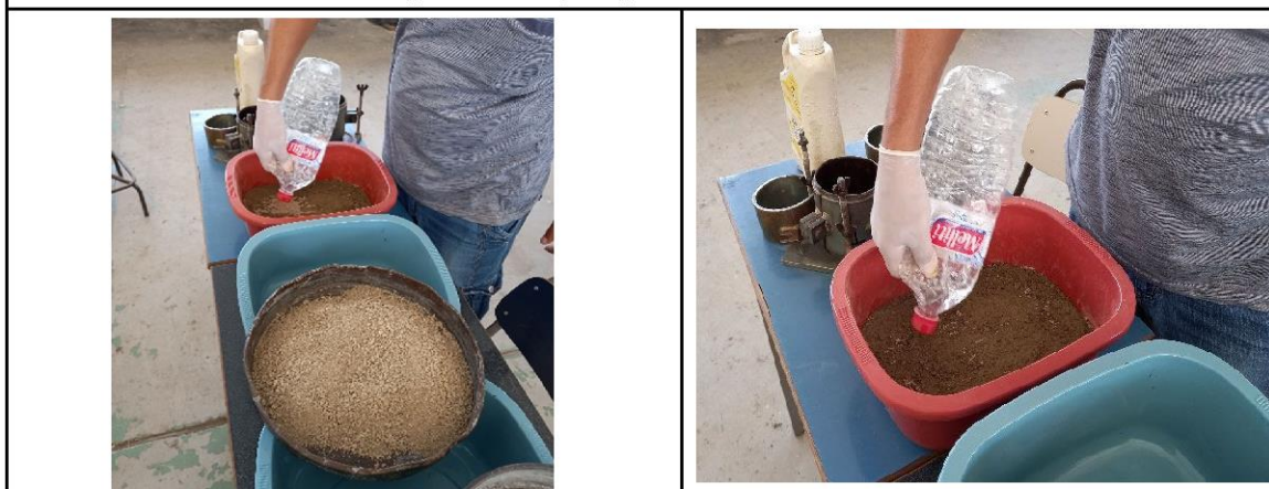
Figure 11. Spraying sediment layers
