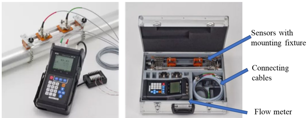
Figure 6-1. External Appearance and Component of Ultrasonic flow meter
