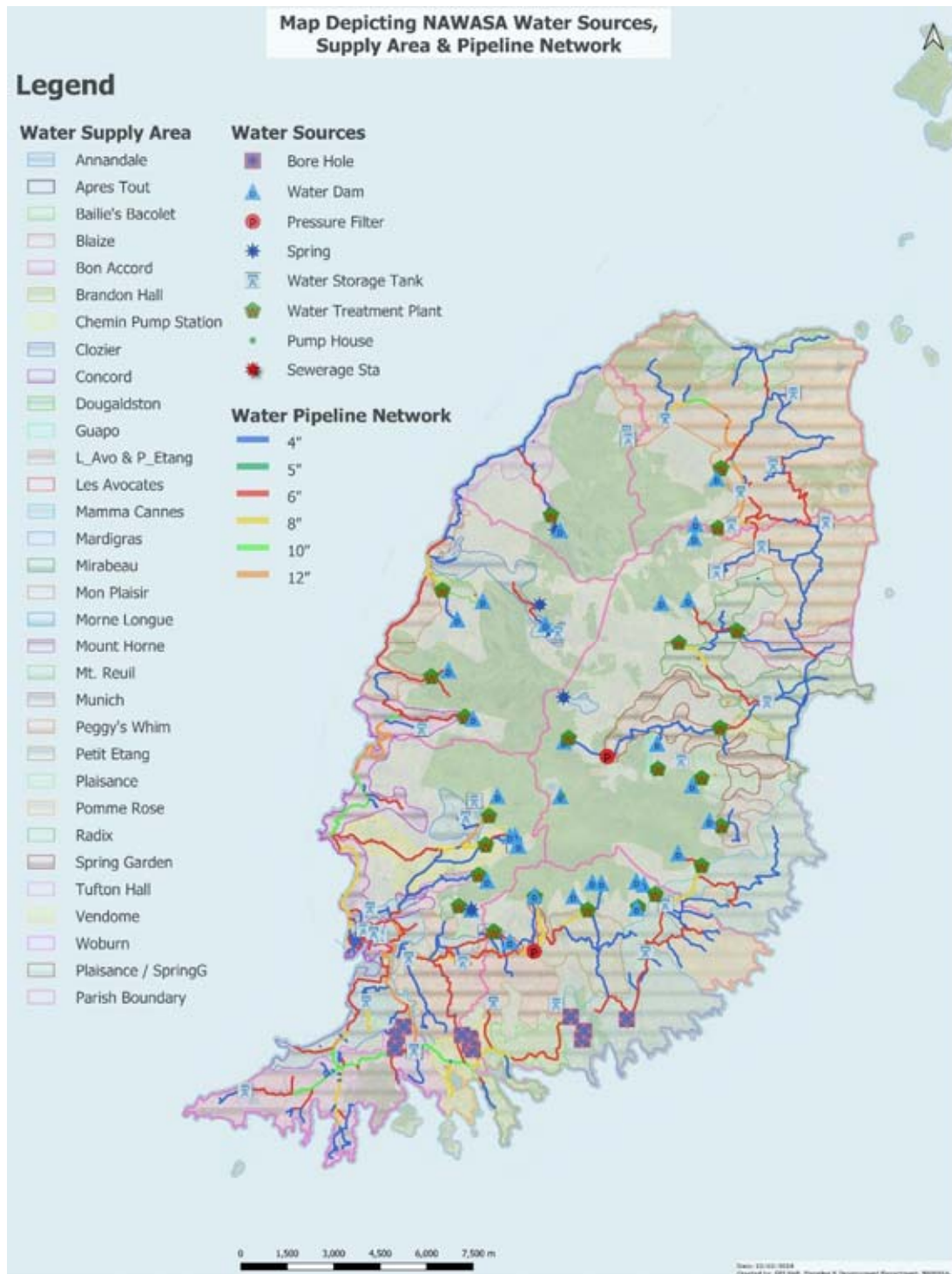
Figure 8-9 Locations of water sources, water supply facilities, and distribution areas of NAWASA
