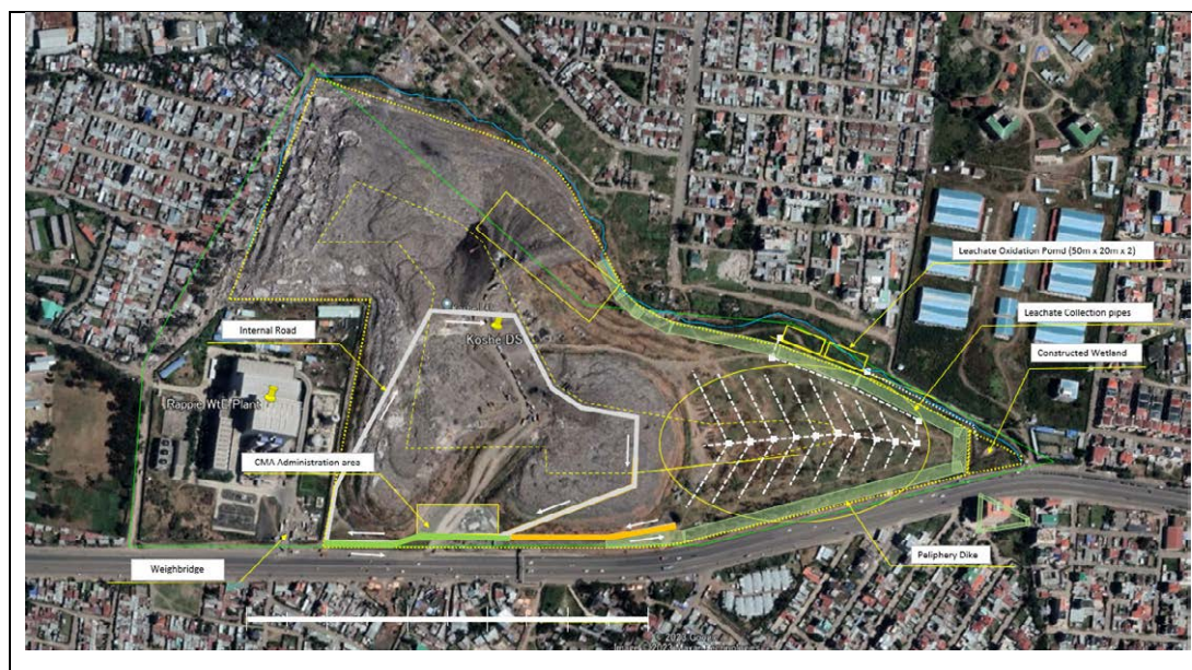
Figure 2-12 Concept for Improving the Koshe Landfill Site by Extending its Life
