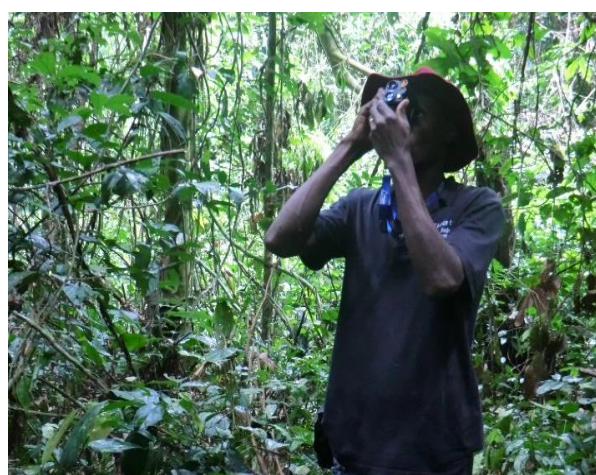
Forest Inventory Training (Height measurement by ultrasound height measuring instrument) (photo: JICA)
