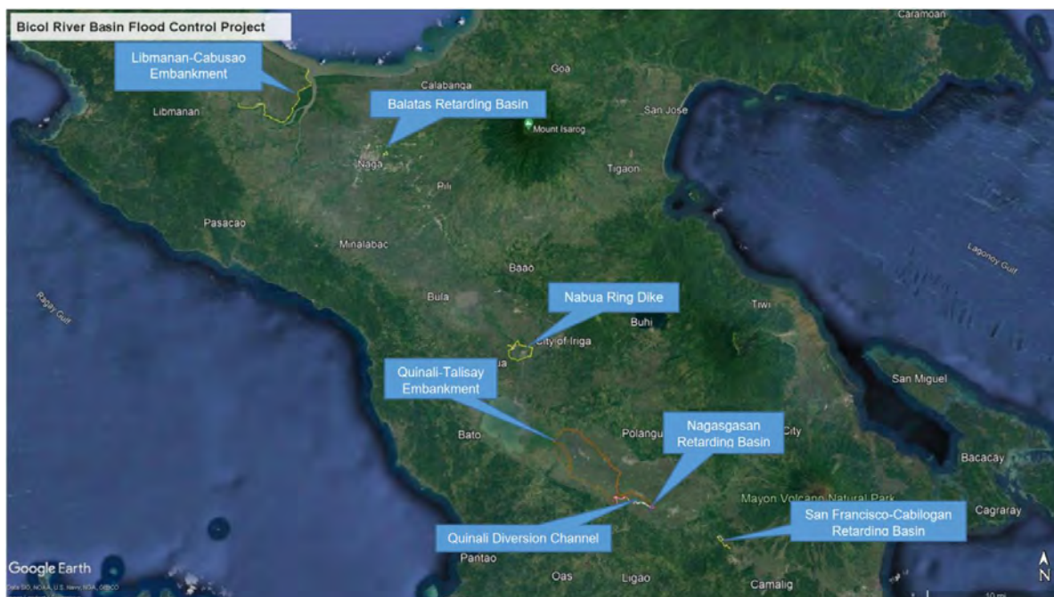
Source: DPWH, The Feasibility Study and Detailed Engineering Design for the Proposed Flood Control Projects in Bicol River Basin, 2022, Project Briefer
