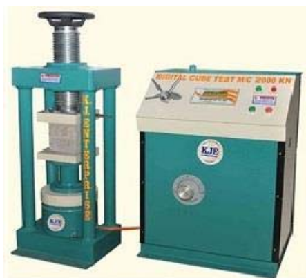
Compression Testing Machine
