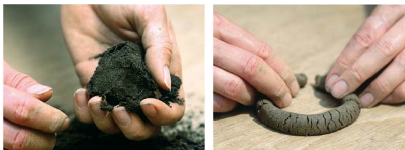
Photo 6-1 Image of soil classification test
