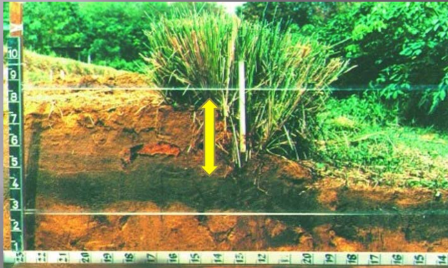
Cross section of a vetiver hedge showing build up of eroded soil after two years. Dark brown layer original top soil. The plant grows up its own created terrace riser. P.K. Yoon Source: Vetiver Network International https://www.vetiver.org/
