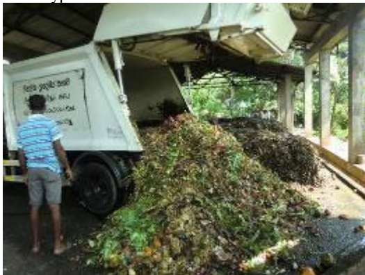
Seethawaka PS Compactor truck with 4-ton capacity donated by WMA. Biodegradable waste is collected by the compactor and transported to a composting facility.
