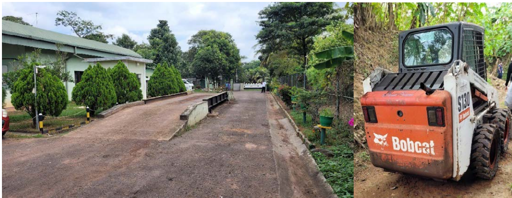
Figure 5 Equipment operated at Kalutara Transfer Station: Truck scale and Bobcat
