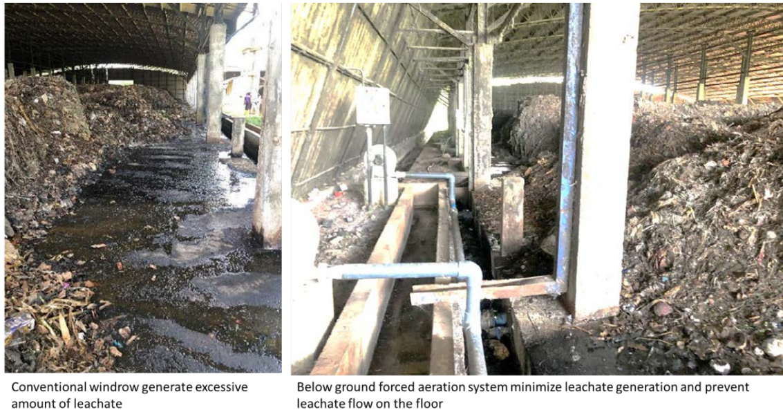
Figure 17 Comparison of leachate generation between conventional windrow and forced aeration system
