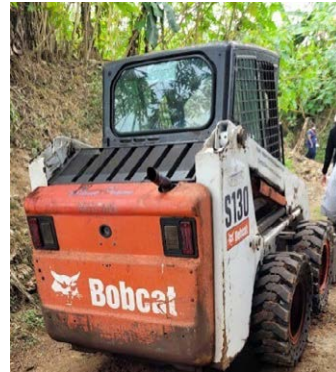
Bobcat used to feed hopped with waste
