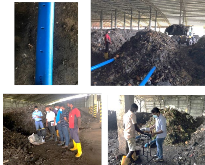
Figure 6 perforated pipe for air supply
